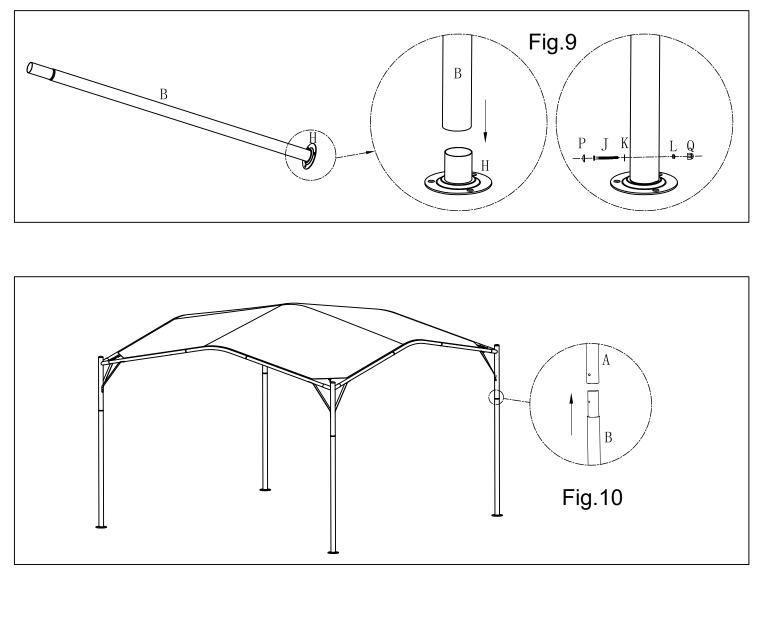
4.1 Attach the Foot Plate H to Post B with hardware P/J/K/L/Q as show in Fig.9. 4.2 Insert the Leg B to the Corner Connector A as show in Fig.10.
