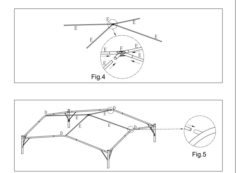
2.1 Insert the Roof Rib E to the Roof Connector F as show in Fig.4.
