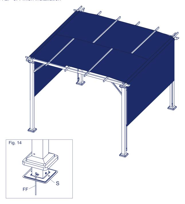
14. Hammer Anchors FF through one of the holes at each post base, into the ground to stablize the gazebo.
